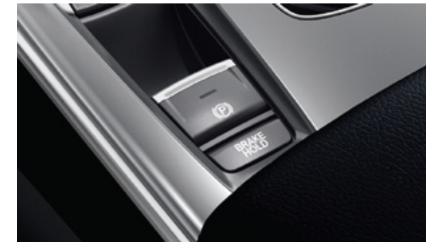
Electric parking brake (EPB) with automatic brake hold
